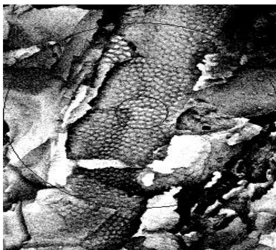
Fig. 9 – SEM showing adsorbent material surface at 400 resolution before treatment
